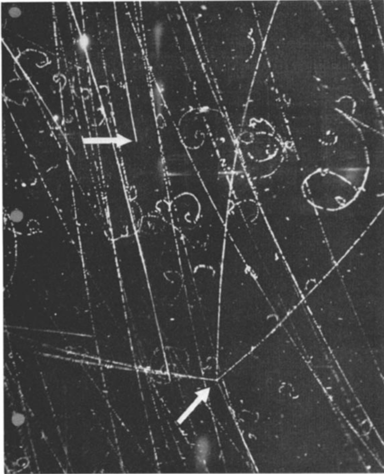
FIG. 12. An antiproton enters a propane bubble chamber, and at the point marked with the upper arrow undergoes charge exchange. The antineutron originates the annihilation star (lower arrow). Density of propane 0.42 \text{ gm. cm.}^{-3} . Real distance between charge exchange and origin of star 9.5 \text{ cm.} T_p at charge exchange \sim 50 \text{ Mev.} From (3).
