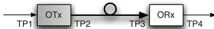
Figure 10. A typical P2P serial digital link system. Signals are checked at test points TP1 to TP4. TP1 and TP2 are at the input and the output of the optical transmitter OTx. TP3 and TP4 are at the input and the output of the optical receiver ORx.
